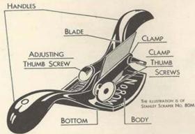
THE CABINET SCRAPER IS USED FOR THE FINAL SMOOTHING BEFORE SANDPAPERING. IT REMOVES THE SUGHT RIDGES LET BY THE PLANE. IT IS ALSO USED TO SMOOTH SURFACES THAT ARE DIFFICULT TO PLANE BECAUSE OF CURLY OR IRREGULAR GRAIN.
